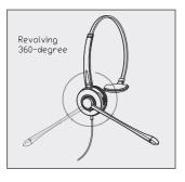
2. To change ears, rotate the microphone boom over the headband to accommodate the left or right ear.
