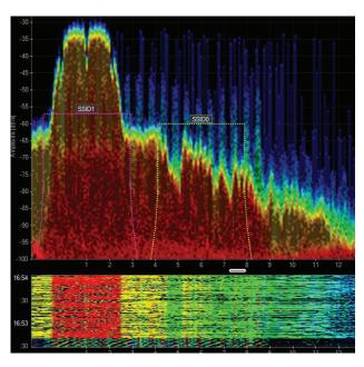
Chanalyzer is designed to bring simplicity and power to the process of wireless troubleshooting. It combines Wi-Spy's ability to read raw RF data with your computer's built-in Wi-Fi card to show you how environmental Wi-Fi saturation and non-Wi-Fi transmitters are affecting your network. Chanalyzer is capable of displaying activity in the 2.4 GHz band, 5 GHz band, or both simultaneously if multiple Wi-Spy devices are present.
