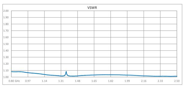
Click the following link (or enter part number in "SEARCH" on website) to obtain additional part information including price, inventory and certifications: Type N F/F Coaxial RF Surge Protector, 800MHz - 2.5GHz, 300W, IP67, 6 V Max., 175uJ, 20kA, Hybrid, Bracket Down, Hole Mount DGXZ+06NFNF-A
