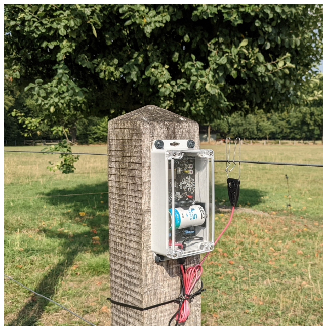
Figure 1: Fencyboy v1.3.1 demo unit with clear cover and single-use battery mounted on wooden fence post.
