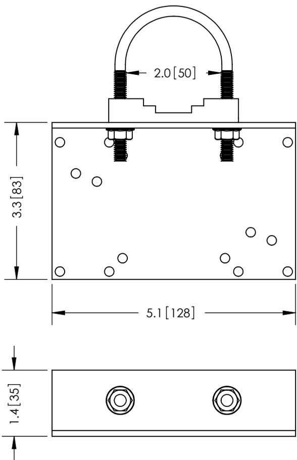
HARDWARE FOR ATTACHING SIGNAL FILTERS AND SPLITTERS INCLUDED
