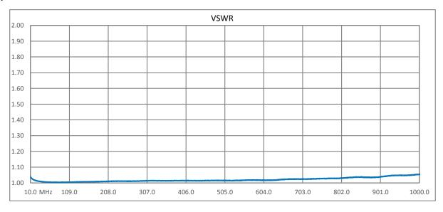
Click the following link (or enter part number in "SEARCH" on website) to obtain additional part information including price, inventory and certifications: Type N M/F Bulkhead Coaxial RF Surge Protector, 10MHz - 1GHz, DC Block, 1.5kW, 3.5mJ, 20kA, Blocking Cap, Hole Mount IS-B50LN-C2-MA
