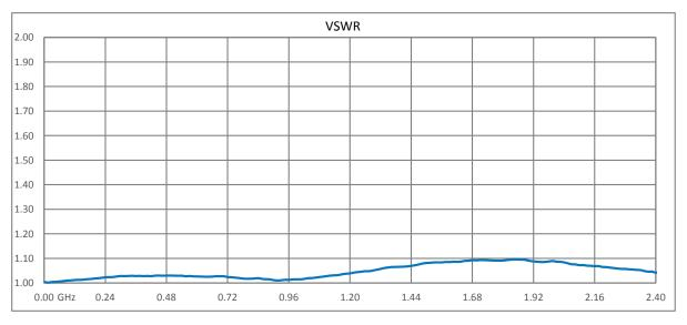
Click the following link (or enter part number in "SEARCH" on website) to obtain additional part information including price, inventory and certifications: Type N F/F Bulkhead Coaxial RF Surge Protector, DC - 2.4GHz, 50W, IP67, 60 V Max., 3mJ, 18kA, Gas Discharge Tube RGT
