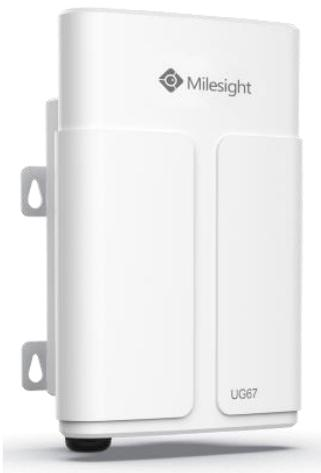
UG67 is a robust 8-channel outdoor LoRaWAN<sup>®</sup> gateway. Adopting SX1302 LoRa chip and high-performance quad-core CPU, UG67 supports connection with more than 2000 nodes. UG67 has line of sight up to 10km and IP67 waterproof case, which is ideally suited to smart agriculture, smart metering and many other outdoor applications.
